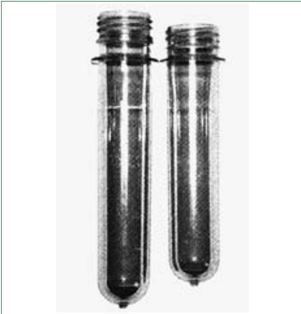
Figura 4: Preforme in PET.
