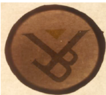
Figure 2. Semi-Transparent 30 \mu\text{m} film 0.4 wt% Loading MWCNT; 6 S/m
