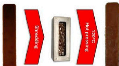
Figure 3. Schematic representation of the thermomechanical recycling of the composite
