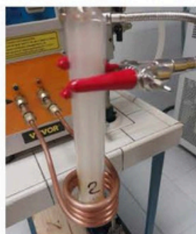
Figure 3. Set-up of induction heating treatment
